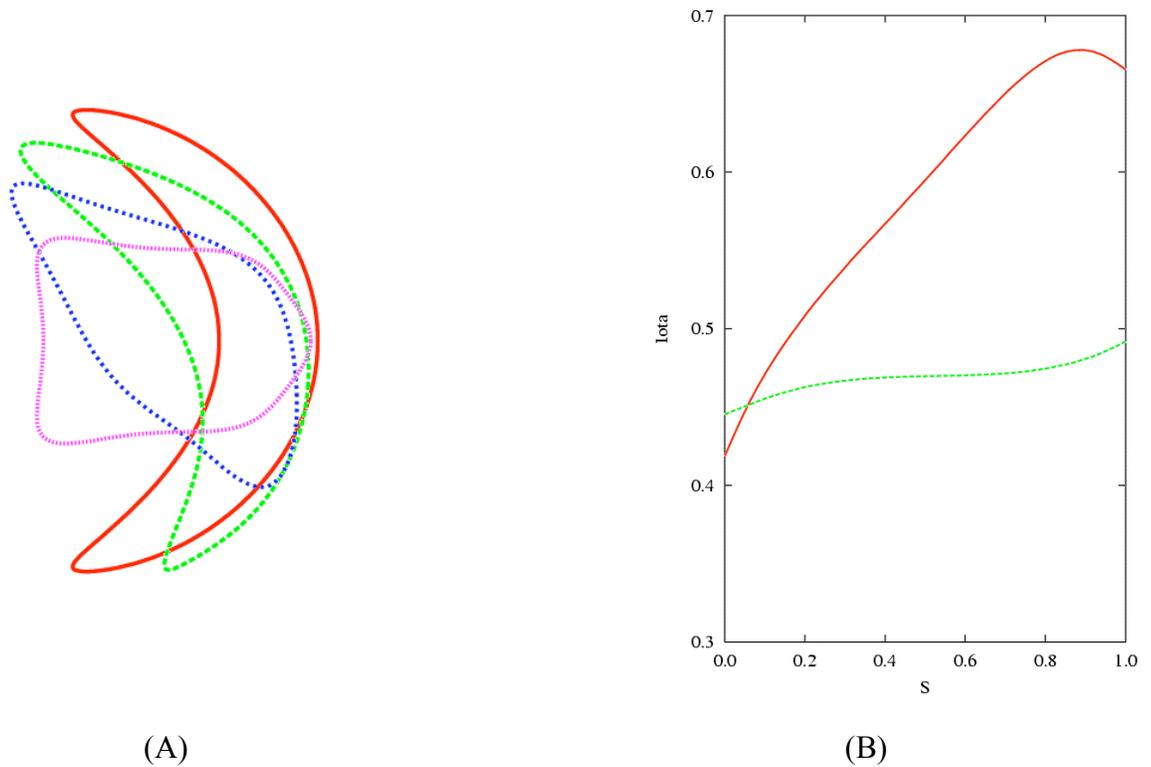
**Fig. 3.** A) Cross section of the LCMS at four toroidal sections and B) the rotational transform as a function of normalized toroidal flux  $s$  for the N3ARE configuration. The dashed line is the rotational transform from external coils (or transform at  $\beta = 0$ ) and the solid line is the total rotational transform (iota) including the bootstrap current contribution at  $\beta = 4\%$ .
