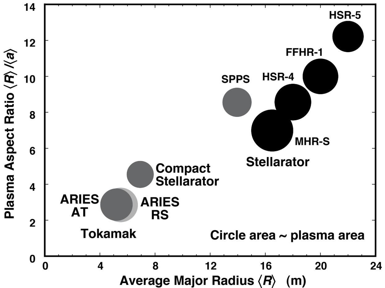
**Fig. 1.** A comparison of size of earlier stellarator power plant studies with more recent advanced tokamak studies, ARIES-AT and ARIES-RS. HSR-5 and HSR-4 are, respectively, 5- and 4-field period Helias configurations. The FFHR is a 10-field period Heliotron/Torsatron ( $l=2$  stellarator) and SPPS is a four-field-period MHH (Modular Helias-like Heliac) configuration.
