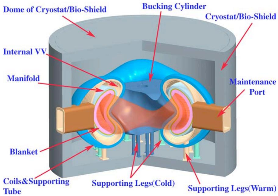
**Fig. 10.** Layout of power plant core showing the coil structure and the maintenance ports.
