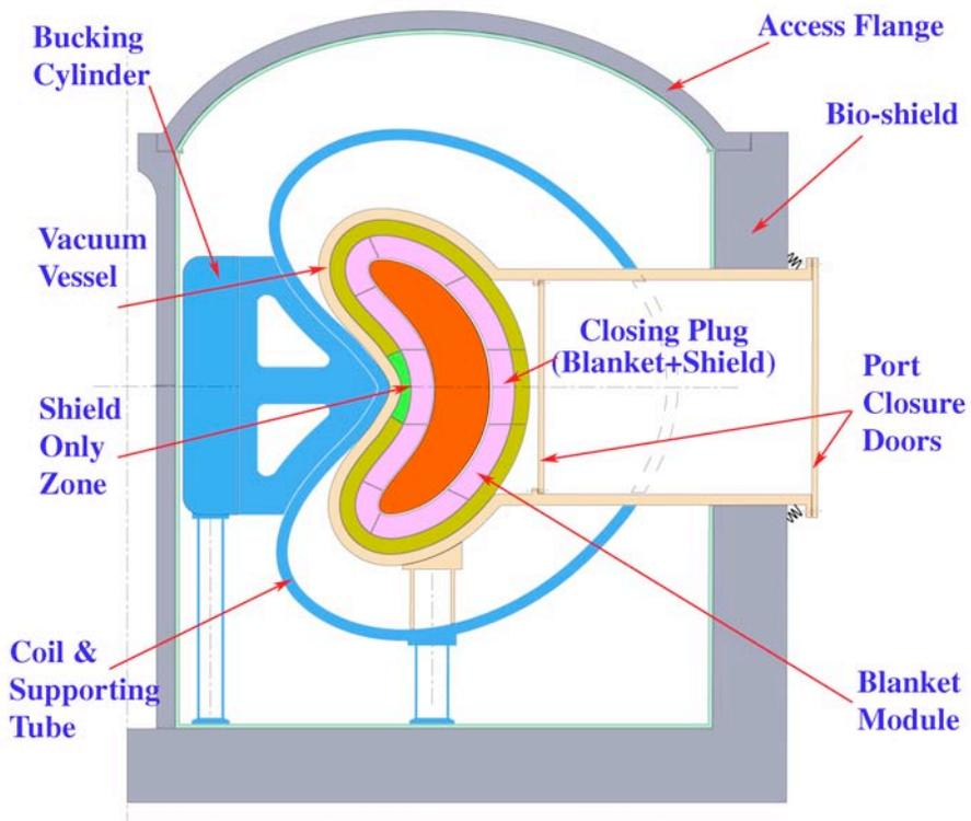
**Fig. 11.** Layout of 3-field period power core for port-based maintenance.
