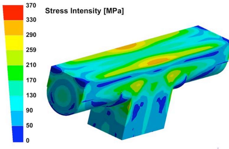
**Fig. 14.** Stress intensity for the basic divertor T-tube layout and a surface heat flux of  $10 \text{ MW/m}^2$ .
