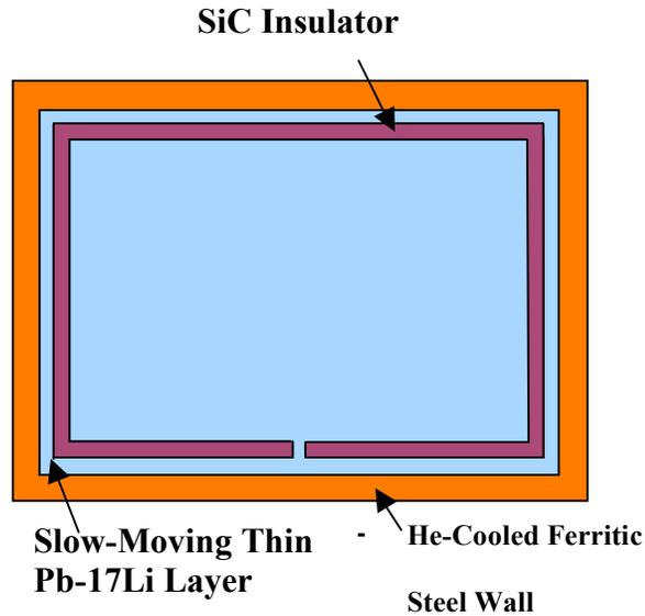
**Fig. 13.** Schematic of SiC layer in inner Pb-17Li channel.
