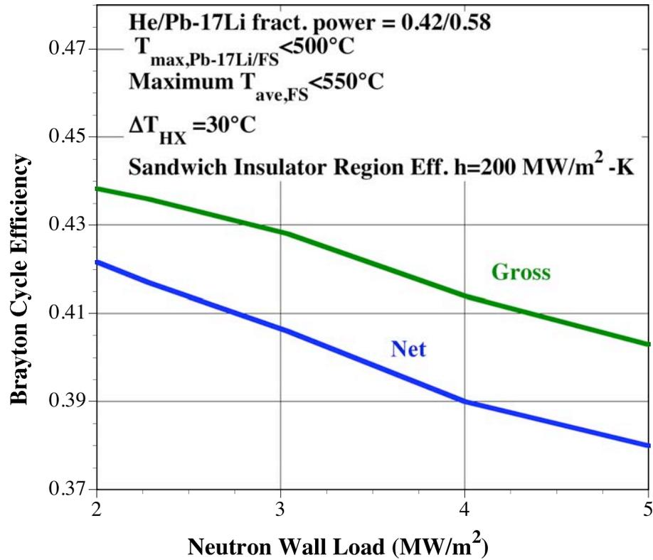
**Fig. 14.** Gross and net (including pumping power) Brayton cycle efficiency as a function of neutron wall load.
