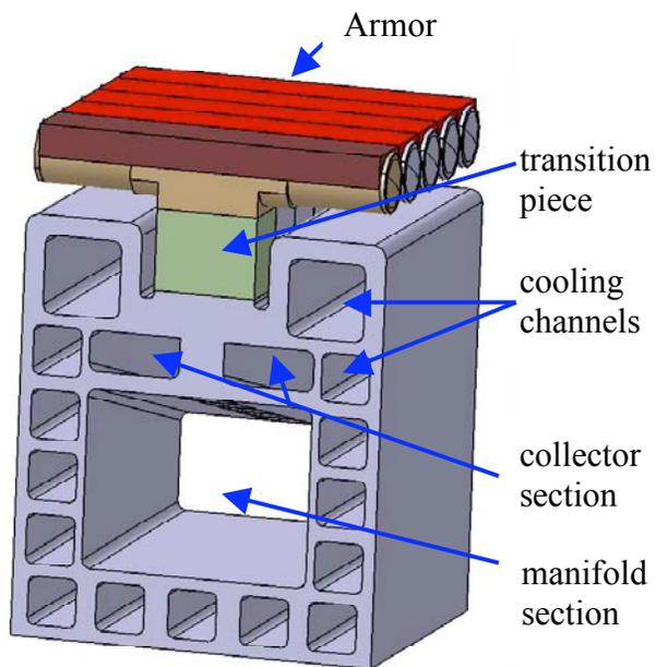
**Fig. 15.** Schematic of divertor target design with T-tubes (tungsten alloy) integrated with coolant manifold made of advanced ferritic steel.
