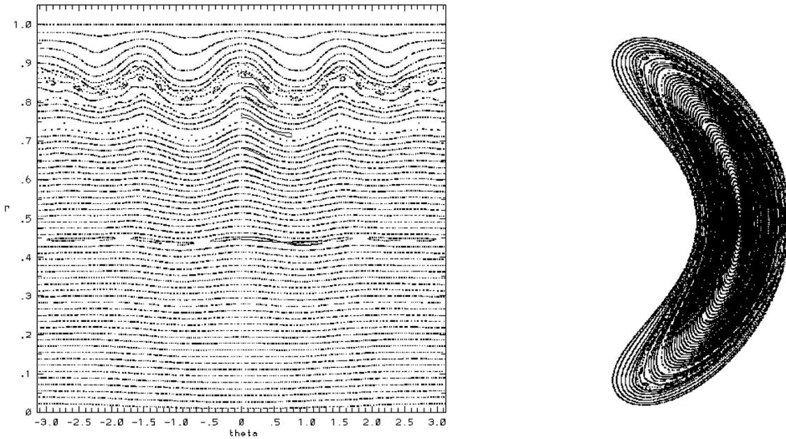
**Fig. 6.** Equilibrium flux surfaces of the KQ26Q configuration as calculated by PIES at  $\beta = 4\%$  showing excellent equilibrium flux surface quality.
