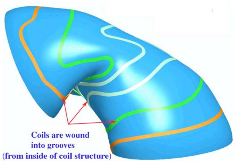
**Fig.15.** Coil structure for one field period showing the location of the winding pack which is wound from inside the coil. Extra structural thickness would be required behind each coil to react the local force (not shown in the figure)
