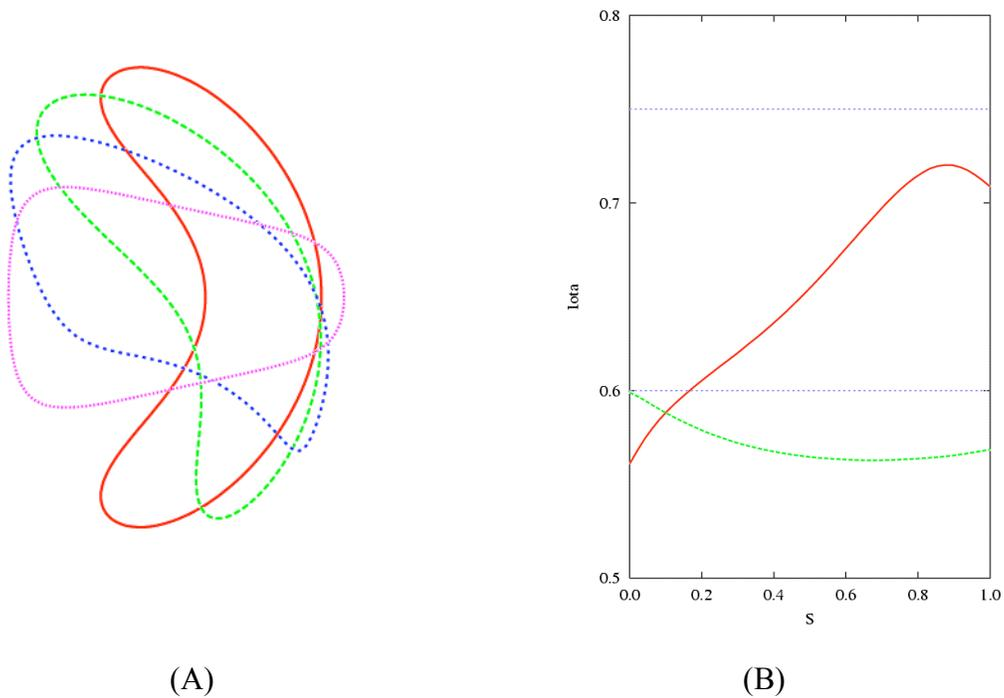
**Fig. 5.** A) Cross section of the LCMS at four toroidal sections and B) the rotational transform as a function of normalized toroidal flux  $s$  for the KQ26Q configuration. The dashed line is the rotational transform from external coils (or transform at  $\beta = 0$ ) and the solid line is the total iota including the bootstrap current contribution at  $\beta = 4\%$ .
