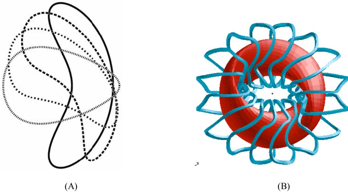
**Fig. 7.** A) Cross sections of the LCMS at four toroidal sections and B) discrete coil designs for the MHH2 configuration (2 field period, plasma aspect ratio of 2.5 [2.7?]).
