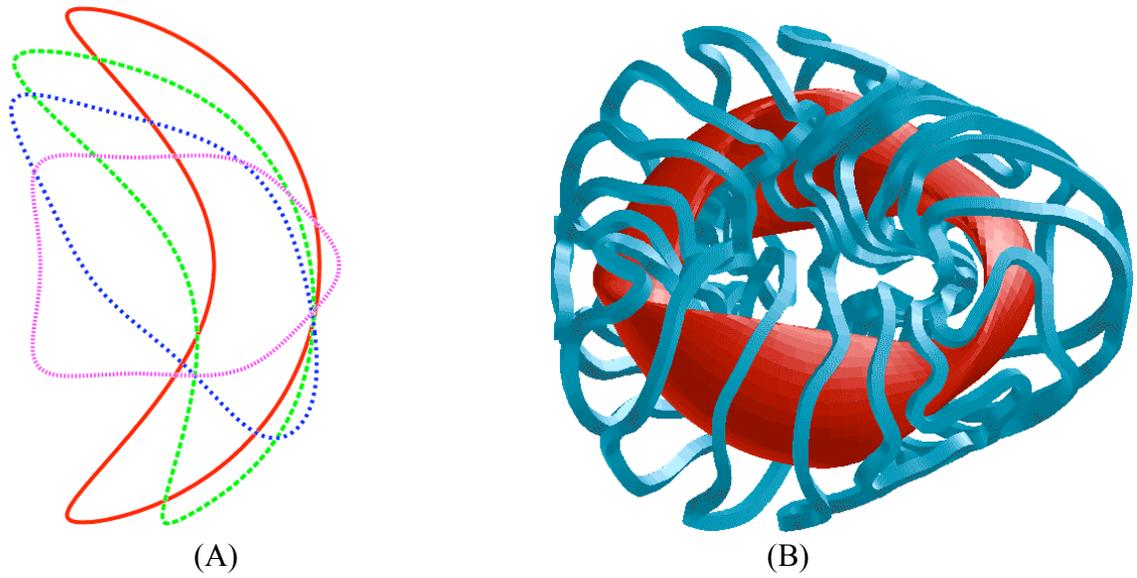
**Fig. 2.** A) Cross section of the LCMS at four toroidal sections for the NCSX-scale-up configuration. B) A typical coil design for this configuration that allows sufficient space between the coils and the plasma.
