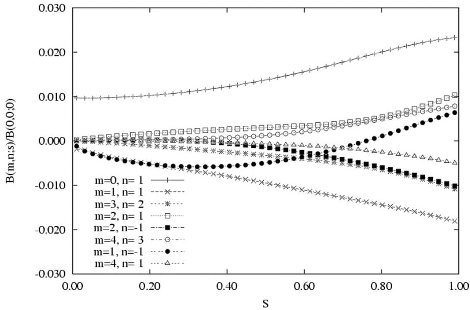
**Fig. 4.** Harmonic contents in the Boozer magnetic spectrum for the N3ARE configuration as a function of the normalized toroidal flux,  $s$ . Note the enhanced  $B(0,1)$  and  $B(1,1)$ , and reduced  $B(2,1)$  and  $B(3,2)$  components.
