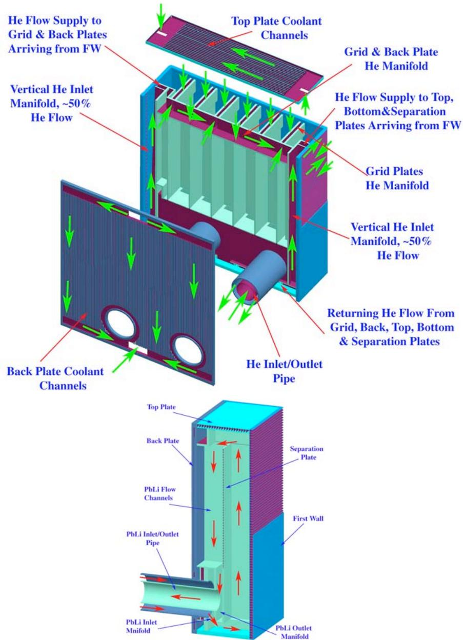
**Fig. 12.** Schematic of He coolant flow in dual-coolant blanket module.
