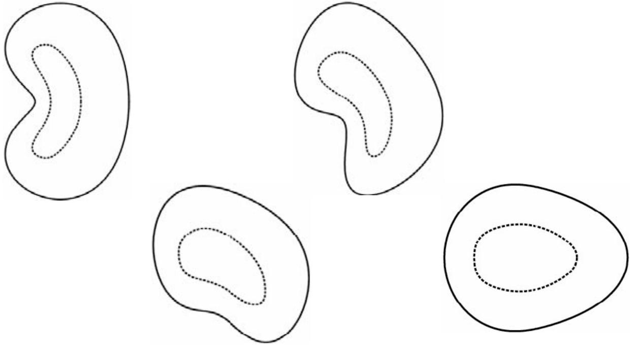
**Fig. 8.** Coil winding surface and the last closed magnetic surface of the MHH2 configuration at four equally spaced toroidal planes over a half-period. The LMCS is found by VMEC at 5%  $\beta$ .
