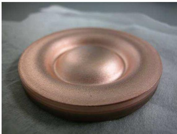
Figure 2.5: Copper sputter target with race track
