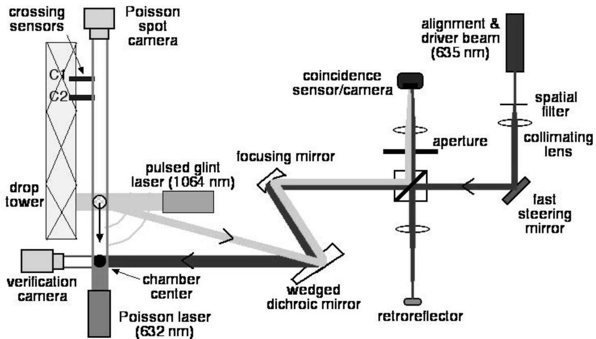
Figure 1. Schematic of integrated target tracking and engagement demonstration. Focusing mirror to chamber center is 2 m, drop tower is ~2 m tall. (Figure not to scale.)
