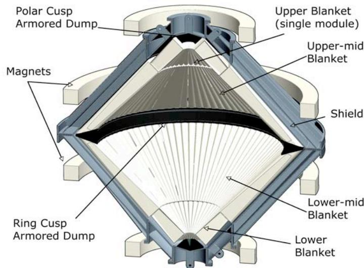
Figure 5. Biconical chamber for simple cusp configuration. [8]
