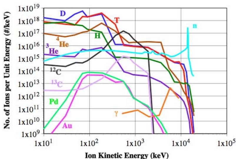
Figure 3. Ion spectra for HAPL 350 MJ direct drive reference target. [4]
