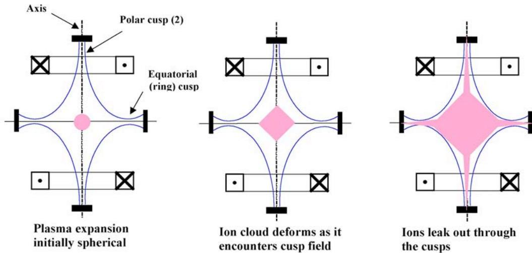
Figure 4. Simple cusp magnetic configuration.
