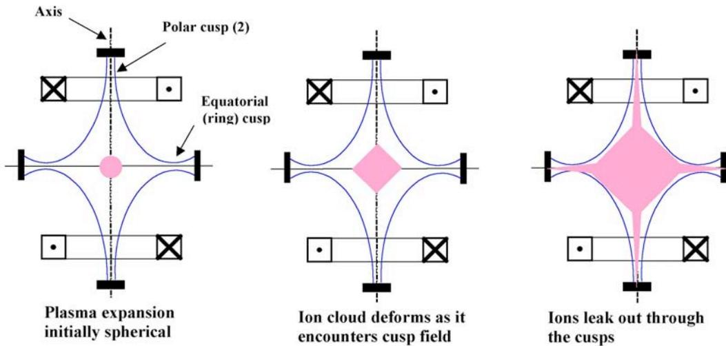
Figure 4. Simple cusp magnetic configuration.
