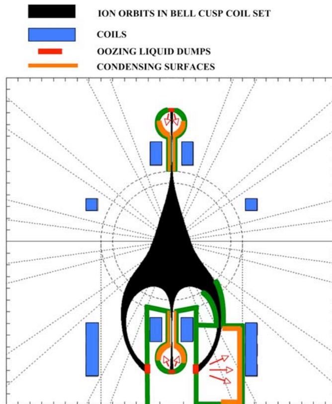
Figure 6. Schematic of bell or tulip cusp showing the ion trajectory through the port, the evaporation from the liquid dump and the condensation surfaces (the scale is in m with a main chamber radius of 5 m). [7]
