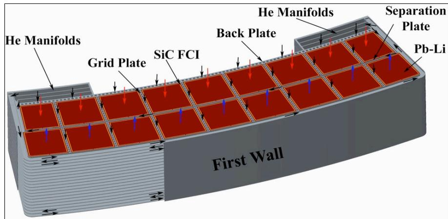
Figure 2. Helium and Pb-17Li flow paths for the ARIES-ACT2 inboard blanket [19]
