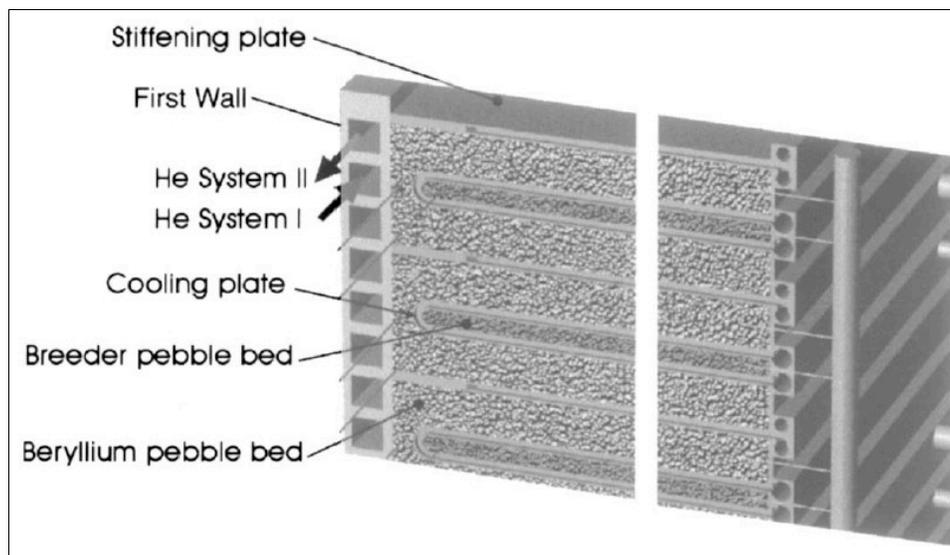
Figure 4. Cross section of the first wall and breeding zone of the HCPB blanket [20]
