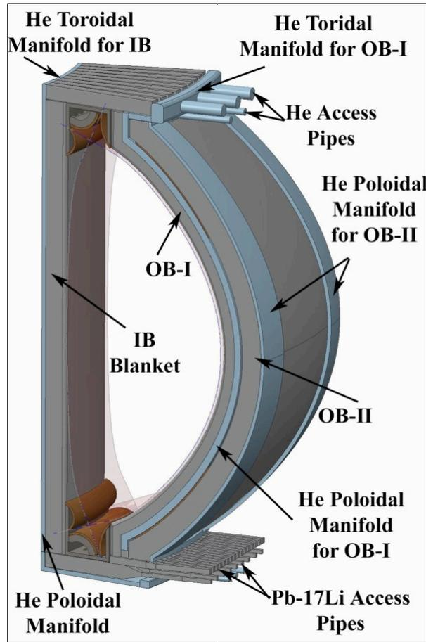
Figure 1. Layout and manifolding for the ARIES-ACT2 blanket [19]
