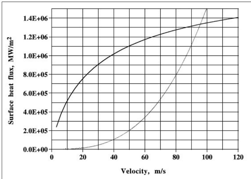
Figure 7. Heat flux window of operation in the ARIES-ST outboard first wall using 5% allowable pumping power [35]
