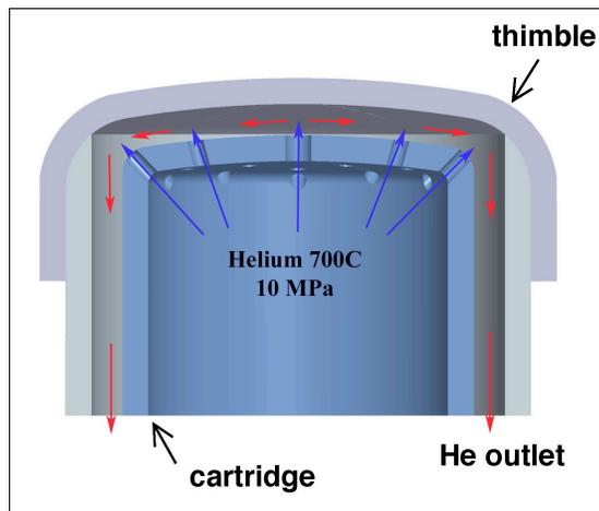
Figure 6. Details of the impinging jets in the finger-type divertor [31]
