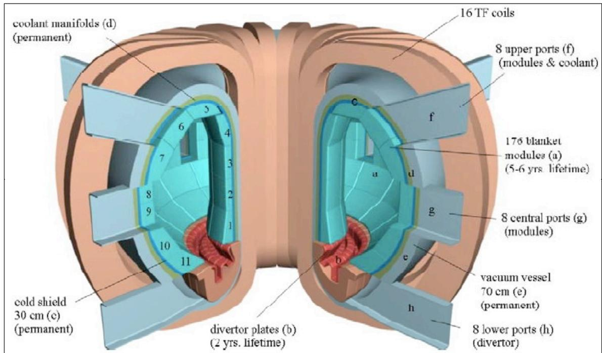
Figure 3. Cut-away view of the fusion power core of the PPCS model C; the other models are broadly similar. [4]
