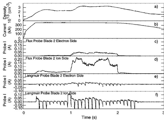
FIG. 6. Typical TEXTOR-94 discharge evolution showing (a) plasma density, (b) plasma current, (c) flux probe current, electron side, (d) flux probe current, ion side, (e) Langmuir probe current, electron side, (f) Langmuir probe current, ion side.
