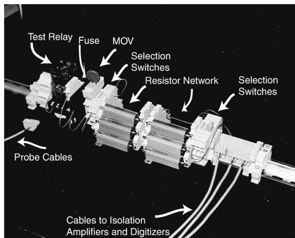
FIG. 5. Photo of a typical modular probe circuit built on DIN modules. All interconnections are not implemented for clarity.
