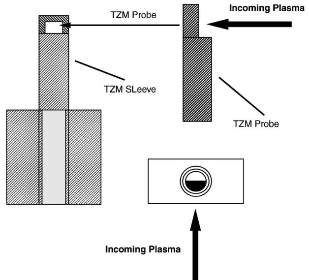
FIG. 3. Schematic of a typical ALT-II probe showing the tungsten sleeve and probe and the alumina insulation.
