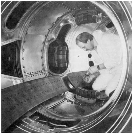
FIG. 1. The inside of the TEXTOR-94 vacuum vessel showing two of the ALT-II blades and the three poloidal limiters.
