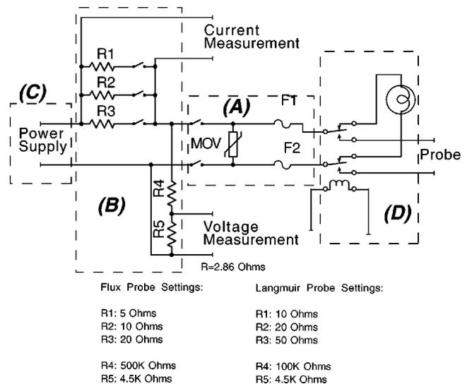
FIG. 4. Schematic of the probe electronics showing the input, current and voltage measurement, B, and the protection and control section, D. The resistor values for the various configurations are noted.
