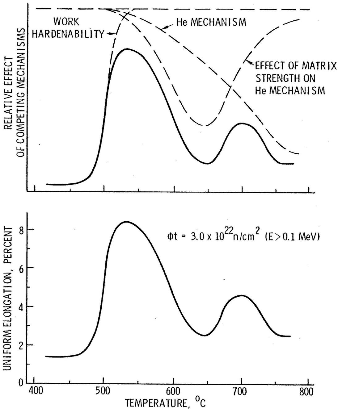
Fig. 8. Effect of temperature on the uniform elongation of irradiated Type 316 stainless steel.
