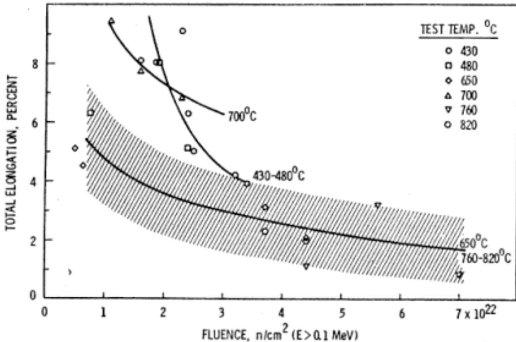
Fig. 2 Effect of fluence on the total elongation of type 316 stainless steel. In EBR-II, 5 dpa  $\square 10^{22}$  n/cm<sup>2</sup>.
