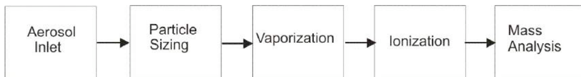
Figure 3- Block schematic for Aerosol Time of Flight Mass Spectrometry.
