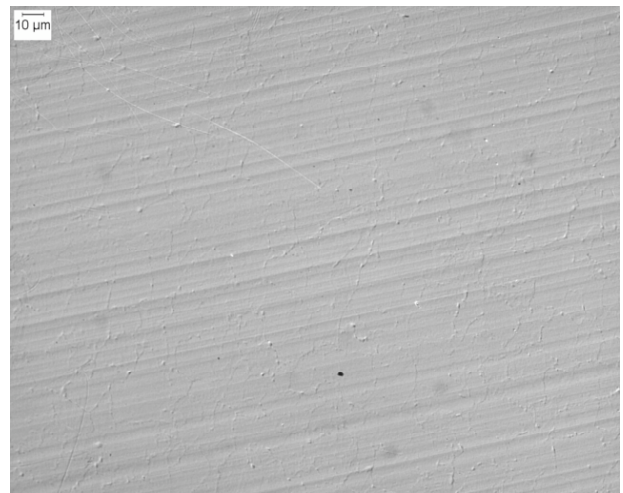
Figure 3. Micrograph of surface electroplated with pure Al, after 10^5 shots at 4 \text{ J/cm}^2
