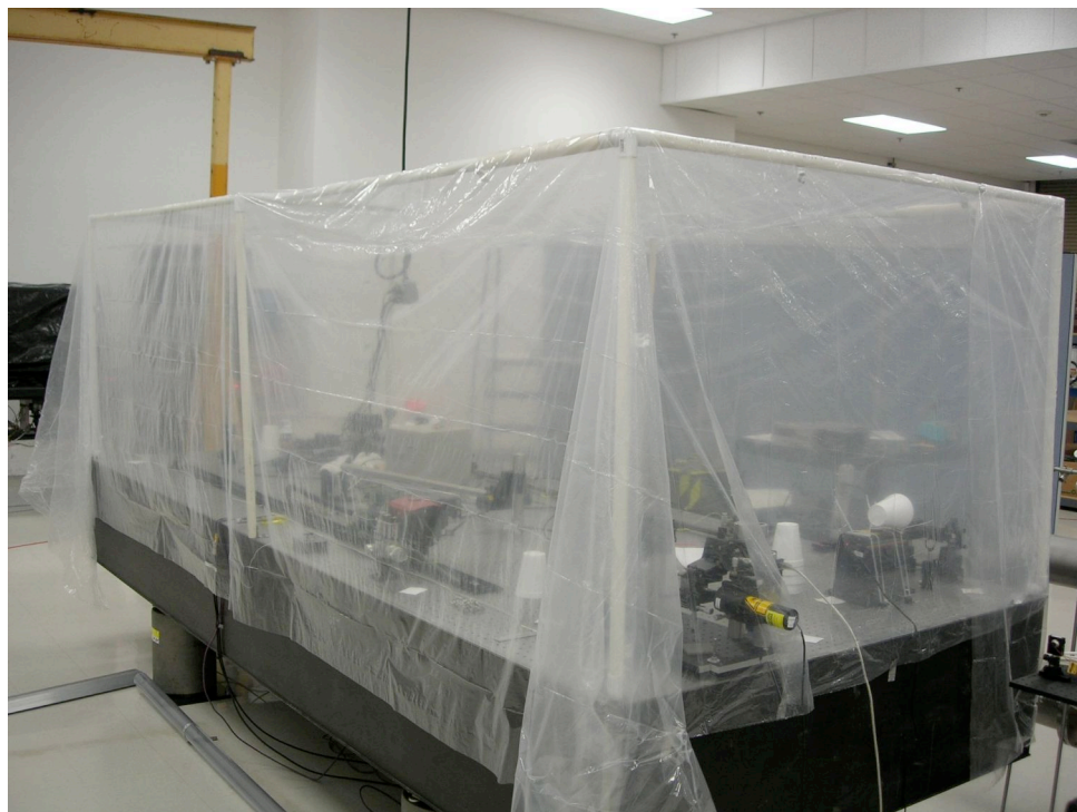
Figure 34 - Plastic tent sheeting used to minimize air currents
