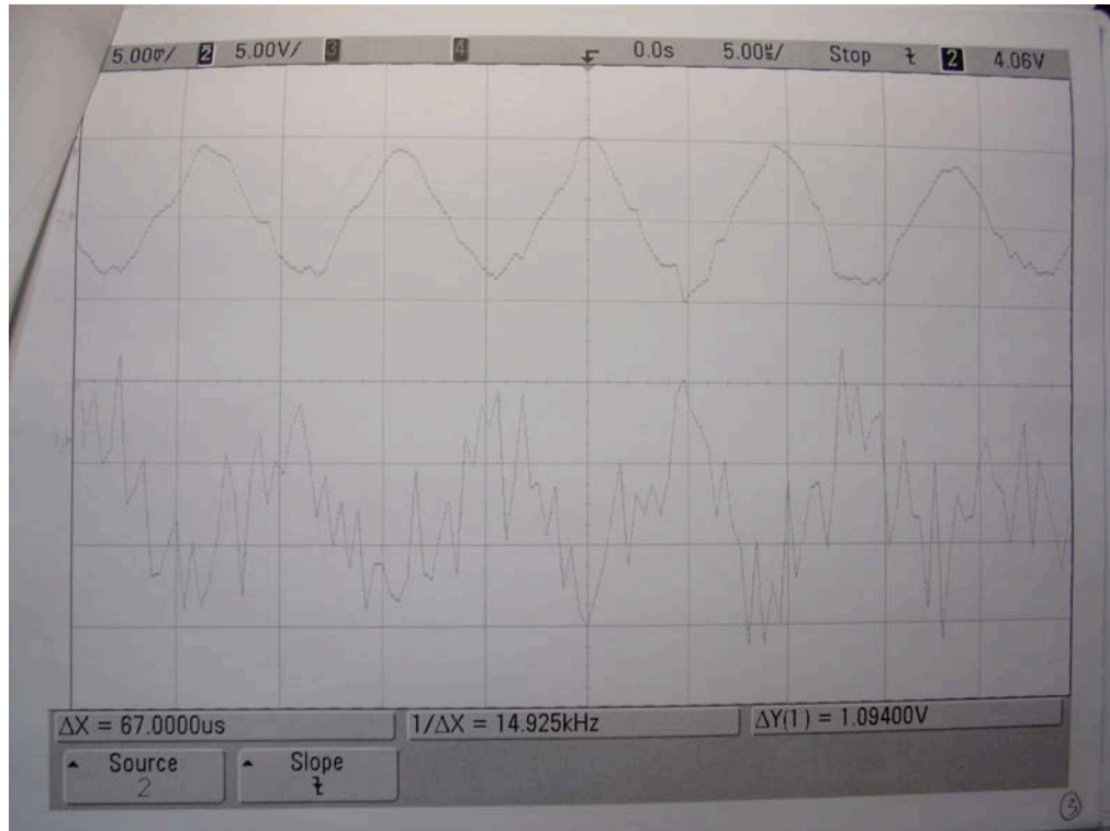
Figure 2.5.4: Demonstration signal results. The top signal has been filtered while the bottom has not (the amplifier/filter inverted the signal). This is the same as the trace in figure 2.5.3, but with a much finer temporal scale. S/N is approximately 3 in the lower trace, and perhaps 10-20 in the upper trace.
