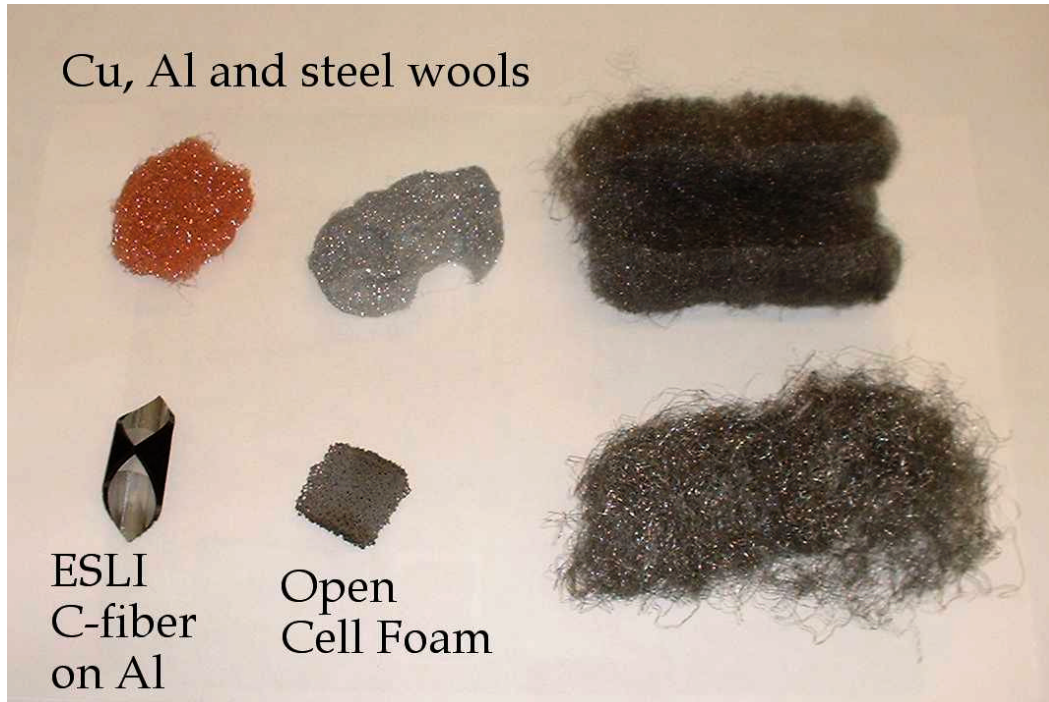
Figure 2. Example of thermal media (ESLI carbon fibers, metal wools, open-cell foam, tailings)
